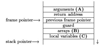
As the reader can see from the figure above, the array and local variables are all below the return address. If an overflow were to occur in the array, nothing important would be overwritten and the overflow would be useless. This also helps with pointers. Take a look at a vulnerable code segment (provided by SSP documentation):
